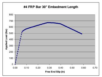
Figure 3. Load-Deformation Behavior of Specimen Reinforced with FRP Bar
